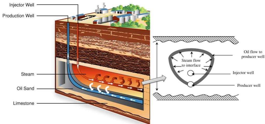
Figure 2: Schematic of the SAGD process ((Hadavand & Deutsch, 2015)).
