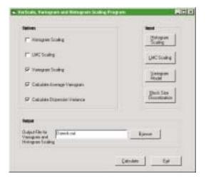
Figure 10: Main window showing the desired boxes checked to accomplish variogram scaling and estimate average variogram and dispersion variance
