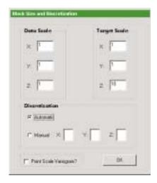
Figure 4: The Block Size and Discretization Window showing the data and target scale along with the discretization option(s) for Histogram scaling example
