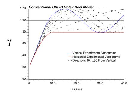
Figure 8: The conventional GSLIB hole effect model at angles 0,..., 90 degrees
