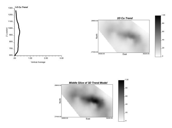
Figure 7: Required 1D trend (left) and 2D trend (middle) for integration to obtain 3D trend (right).
