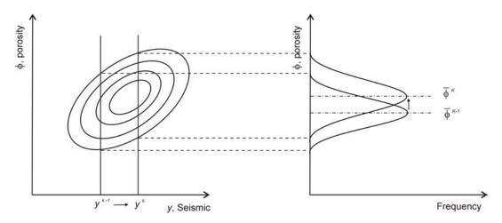
Figure 1: Schematic illustration of how seismic affects porosity
