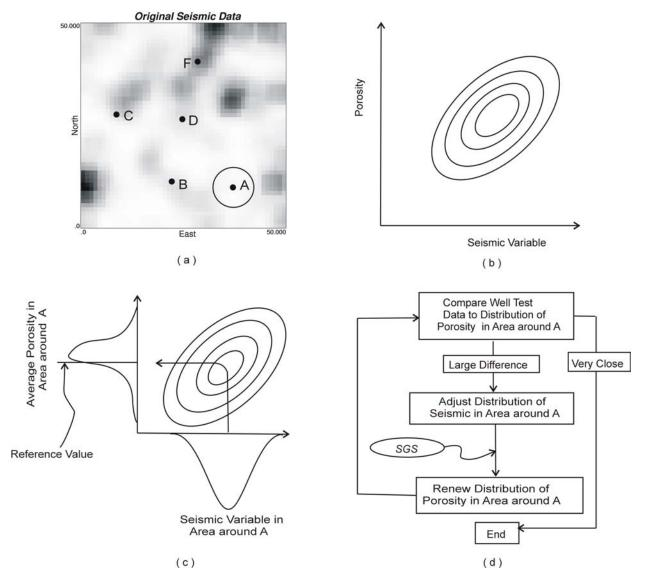
Figure 2: Schematic illustration of methodology
