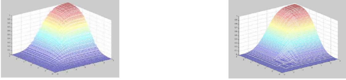
Figure 4: 3-dimensional surface plots of reference (left) and estimated (right) joint cdf for bivariate Gaussian case.
