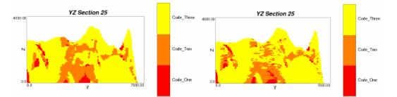
**Figure 11:** The facies models with different Z grid definitions. The left facies model is built with 100 Z grids; the right facies model is built with 500 Z grids. More geological details can be revealed with fine grid definition, and the facies continuity is better too.
