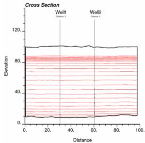
**Figure 14:** The E-type mean surface model of 99 unconditional Surfsim realizations. The total surface number is 20 and the volume to fill is set to 0.90.
