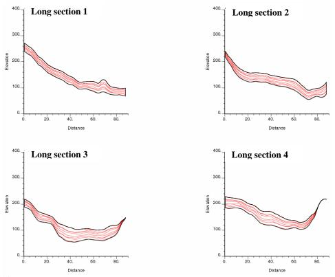
**Figure 13**: Some long sections of the synthetic boundary surfaces example. Both bounding surfaces are flattened to honor proportional stratigraphic correlation, and the number of surfaces is well selected to meet this need.
