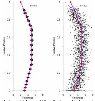
**Figure 15:** Comparing the layer thickness of 99 realizations with the trend definition. The standard deviation for each layer is set to 0.1 on the left plot, and it is set to 1.0 on the right plot
