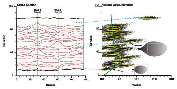
**Figure 8:** Vertical trend analysis of one surfsim realization of conditional run. The surfsim program used here is the original version. Note that the well conditioning data control the vertical volume trend distribution. Also note that the generated surface geometry is very large, so no surfaces stacking pattern will be honored.
