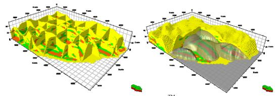
**Figure 23:** The fence view of the facies model from  $Petrel^{TM}$ . **Figure 24:** The cut view of the facies model from  $Petrel^{TM}$ . Some surfaces are plotted to check the facies distribution in lobes.
