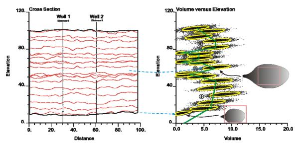
**Figure 9:** Vertical trend analysis of one surfsim realization of unconditional run. The surfsim program used here is also the original version. Note the four vertical volume trend cycles. Also note that the generated surface geometry is very large, so no surfaces stacking pattern will be honored.
