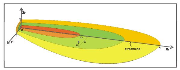
**Figure 4:** Idealized facies distribution of a turbidite lobe. This plot also shows how to locate the 3D relative position of a given cell within a turbidite lobe (after M.J. Pyrcz, 2003). The scale of this lobe is equivalent to the 2<sup>nd</sup> order turbidite lobe defined by M.J. Pyrcz (2003).
