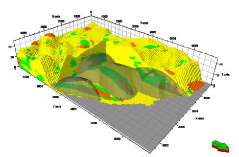
**Figure 19:** The cut view of the facies model from Petrel<sup>TM</sup>. Some modeled surfaces are also plotted to check the facies distribution in lobes.
