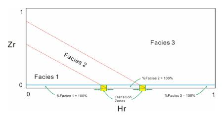
**Figure 7:** The facies transition zones of Model I. It is clear that the transitions are very narrow for any facies model using Model I, which means that the facies realizations will be very similar on the base surface for a given lobe.
