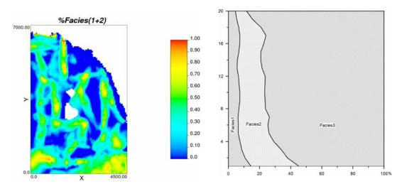
**Figure 21:** The NTG map of the facies model and vertical facies proportion. Facies 1 and 2 are treated as net facies in this case.
