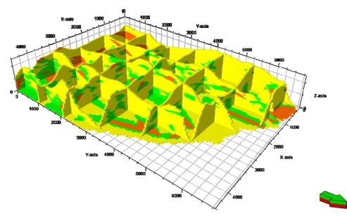
**Figure 18:** The fence view of the facies model from Petrel<sup>TM</sup>. The curvilinear shape can be visualized clearly, and the facies model is very clean.
