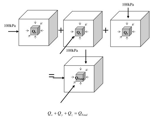
**Figure 5:** Calculation of the total flow rate in a block for three pressure gradients.
