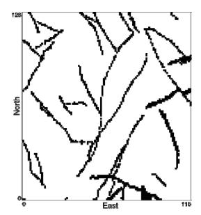
**Figure 2:** Typical horizontal slice of the Whiteshell fracture model. Originally the fractures are planar features described by triangular facets but have been rasterized into a block model.
