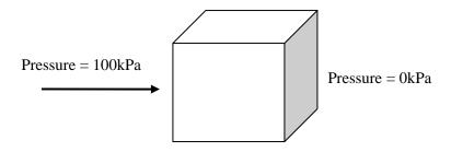
**Figure 3:** Pressure gradient in the *x*-direction with the box representing the 3D fracture model.
