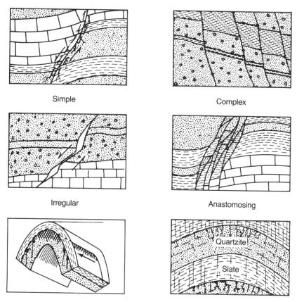
Figure 1: Types of basic folding and faulting (Guilbert and Park, 1996)
