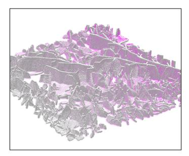
**Figure 6:** View of the fracture model. Fractures are shown in gray, the host rock is transparent.
