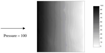
**Figure 7:** Slice of pressure with a horizontal pressure gradient generated from FLOWSIM (Deutsch, 1987).
