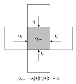
**Figure 4:** Calculation of the total flow rate in a single block (gray block) in a 2D fracture model.
