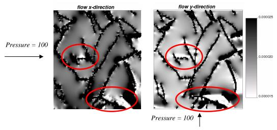
**Figure 8:** Total flow in the model for pressure gradients in the x and y directions.
