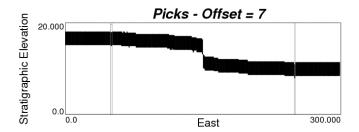
Figure 13: An example of the output produced by pickselplt showing both a coal seam and the drill holes.
