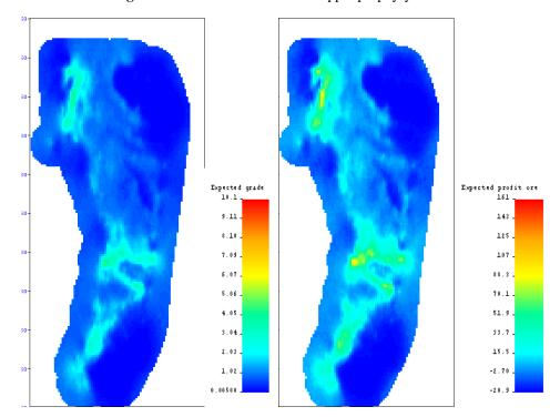
Figure 4: E-type copper model and model of expected profit.
