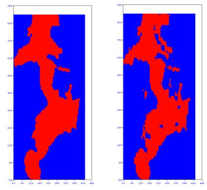
Figure 6: The results of dig limit and feasibility grade control compared. It is easily seen that they are very similar.
