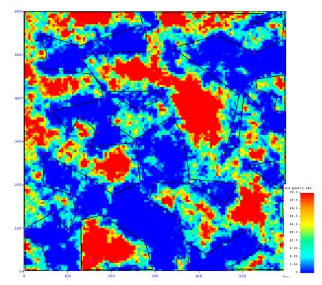
Figure 7: Expected profit model with initial dig limits for a second example.
