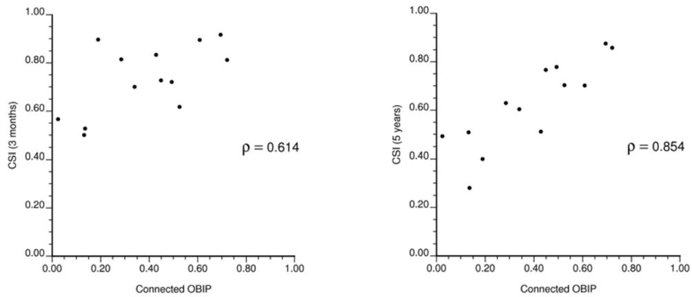
**Figure 10:** Cumulative steam injection versus the connected OBIP ranking at 2 stages during the flow simulation.
