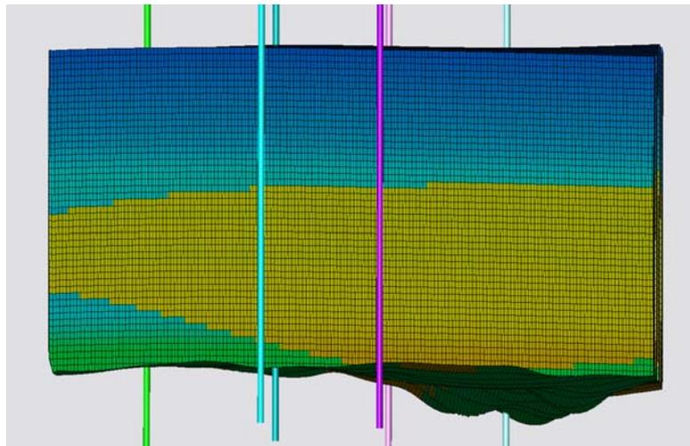
Figure 1: Basal unconformity for a local grid.
