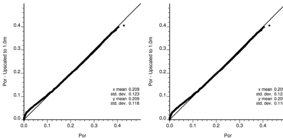
Figure 2: Q-Q plots of the upscaled porosity.
