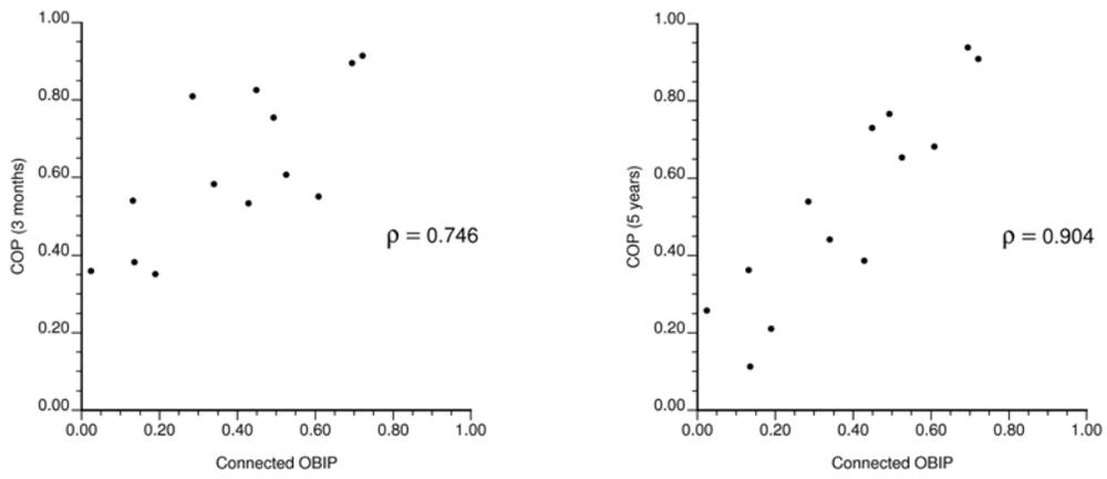
**Figure 9:** Cumulative oil production versus the connected OBIP at 2 stages during flow simulation.
