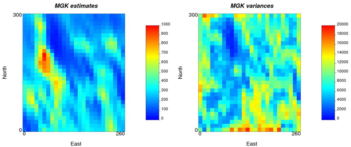
**Figure 9:** Traditional multiGaussian Kriging block estimates (left) and variances (right).
