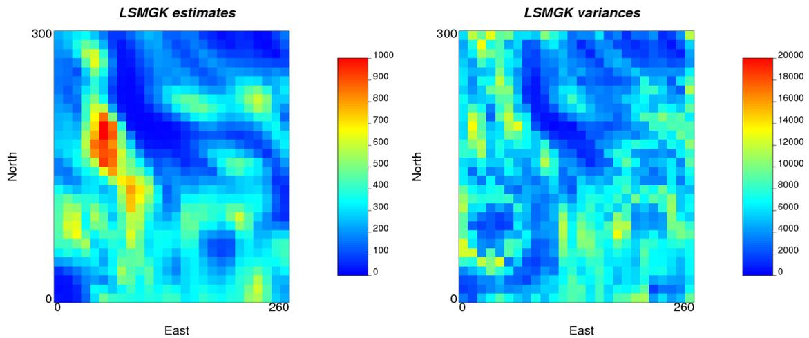
**Figure 10:** Locally stationary multiGaussian block estimates (left) and variances (right).
