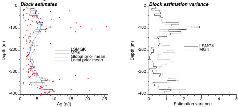
**Figure 6:** MGK and LSMGK block estimates (left). MGK and LSMGK block variances (right).
