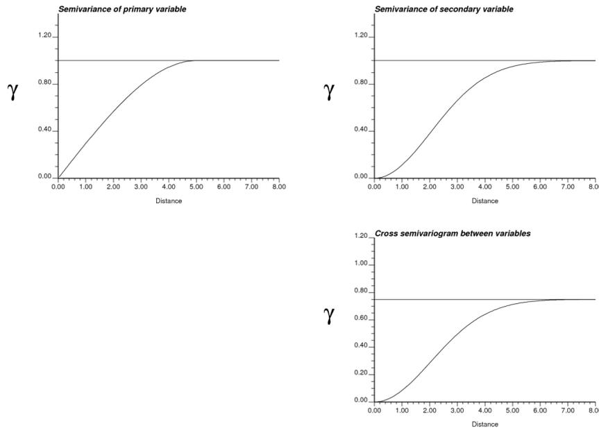
**Figure 2:** Theoretical example of a generalized Markov model of coregionalization given in (25) with a high correlation coefficient  $\rho = 0.75$ .
