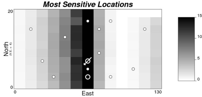
**Figure 3.** Map of average sensitivity coefficient and location of 12 selected master points (white dots).
