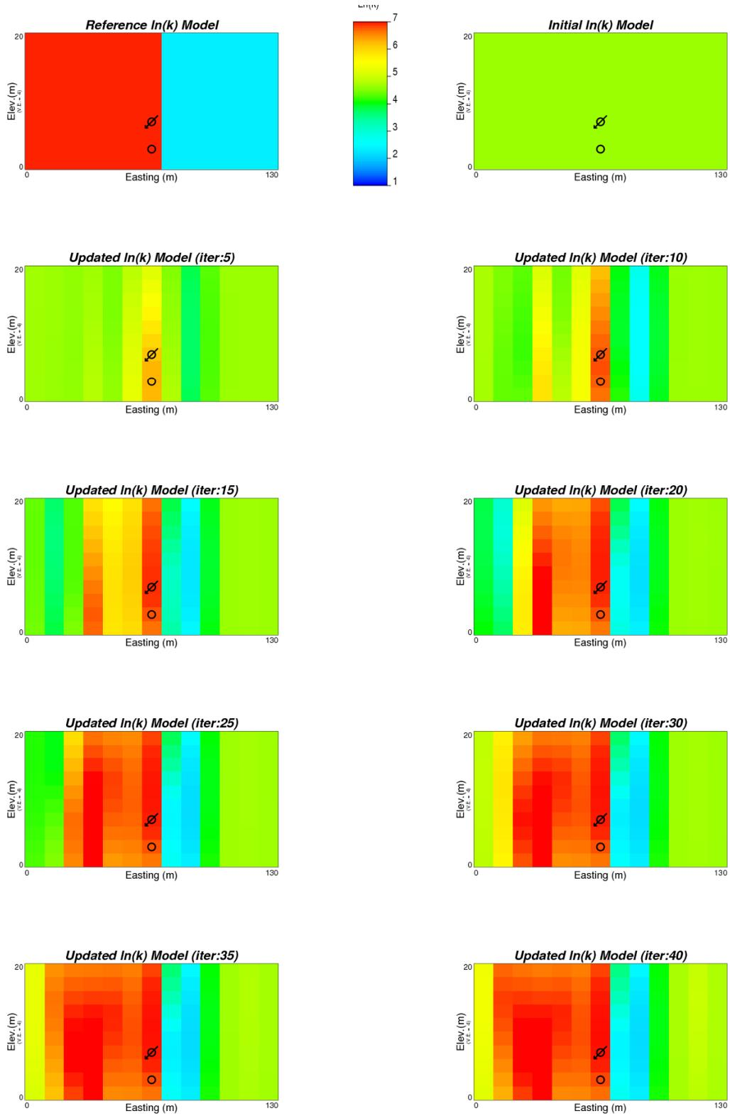
**Figure 6.** Reference Permeability Model (top left), Initial Permeability Model (top right) and Eight Updated Permeability Models.
