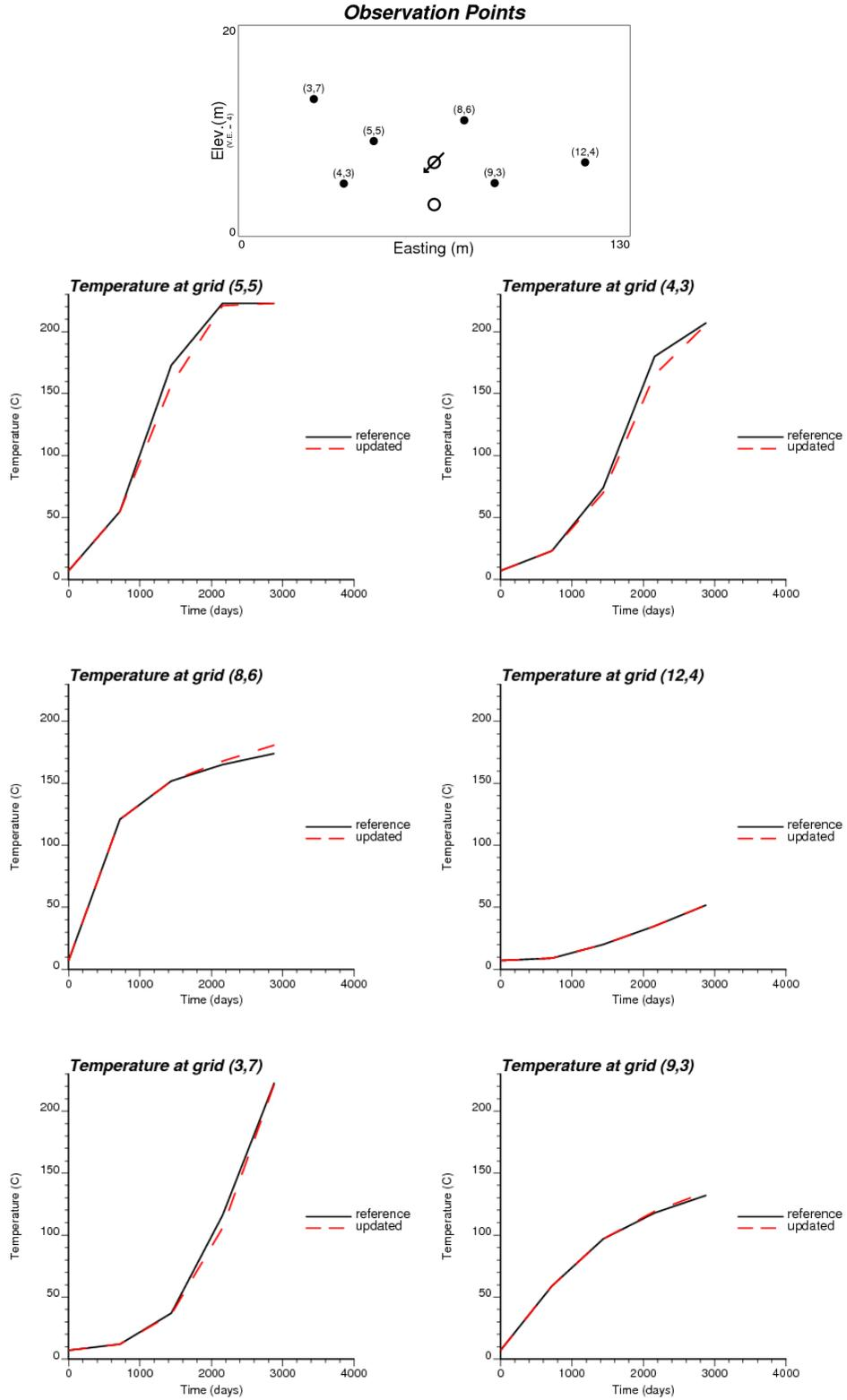
**Figure 8.** Location of observation points (top) and the temperature responses computed from the updated permeability model (dash line) and reference temperature response (solid line) at observation points.
