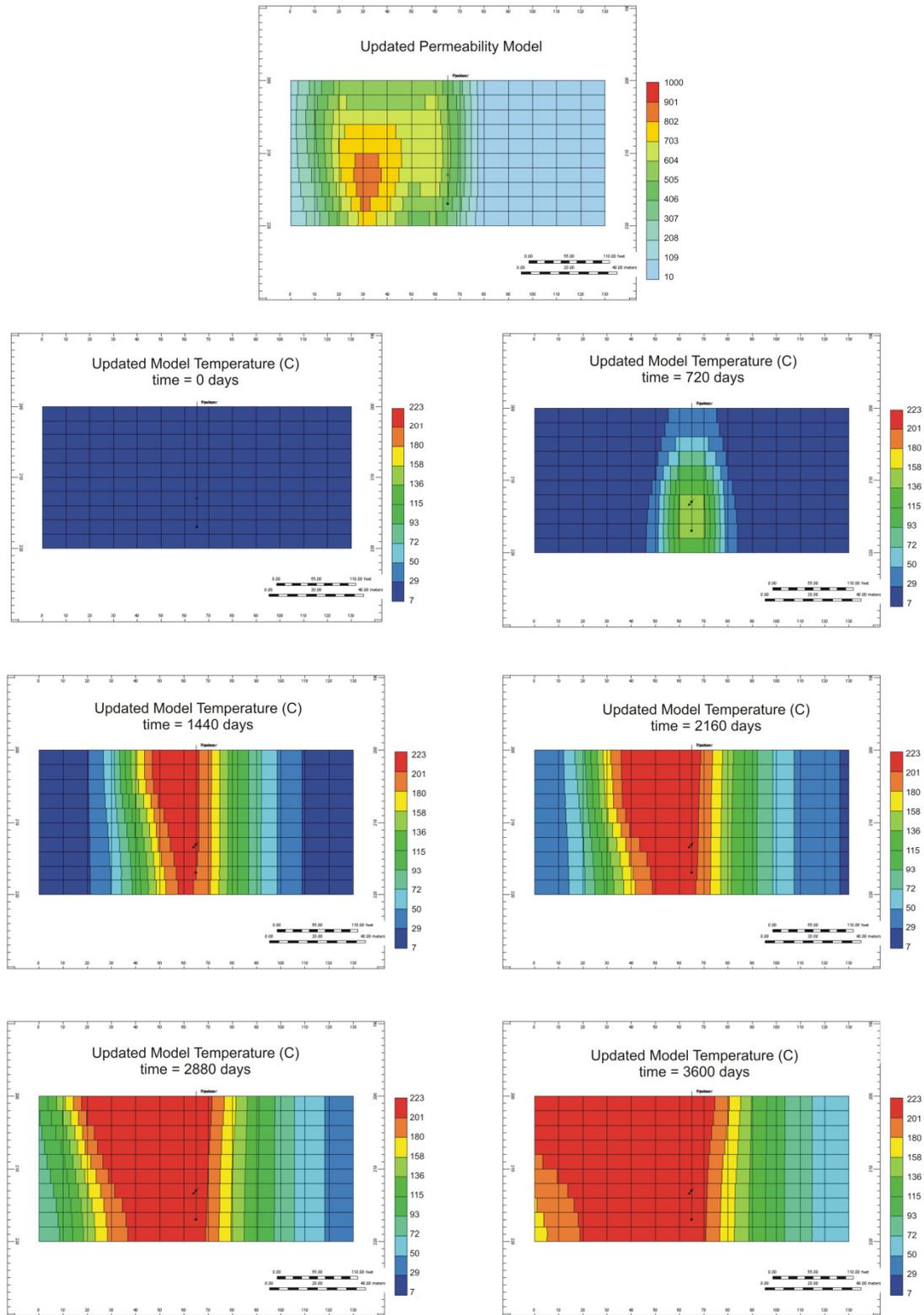
Figure 7. Updated Permeability Model (top) and Temperature Responses at Five Time Steps.
