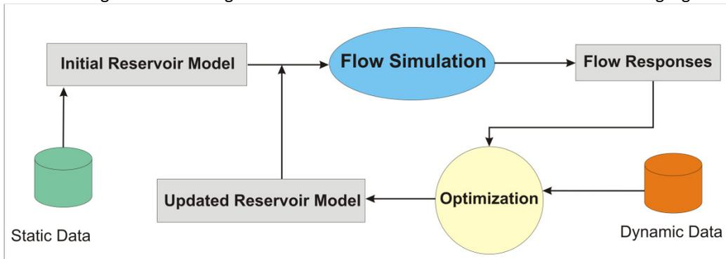
Figure 1. Typical Reservoir Modeling Workflow.
