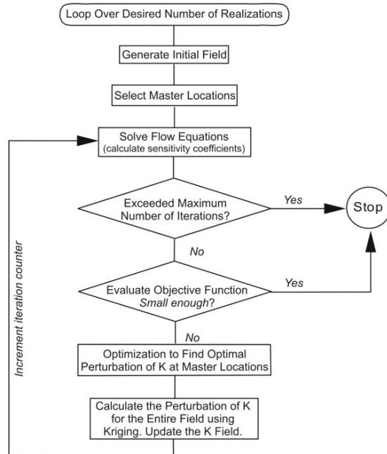
Figure 2. Flowchart of the Sequential Self Calibration (SSC) Method (Wen et al., 2005).
