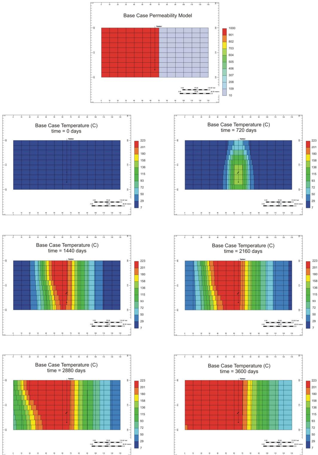
Figure 5. Base Case Permeability Model (top) and the Temperature Responses at Five Time Steps.
