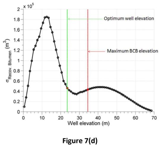
**Figure 7:** Result in case of a rough BCB surface **(a)** well elevation Vs recoverable bitumen from 100 realizations, a rough BCB surface. **(b)** Realization # 1, and optimal well placement. **(c)** Optimum well elevation and maximum BCB elevation from output of realizations. **(d)** Measure of uncertainty of well depth in terms of recoverable resource.
