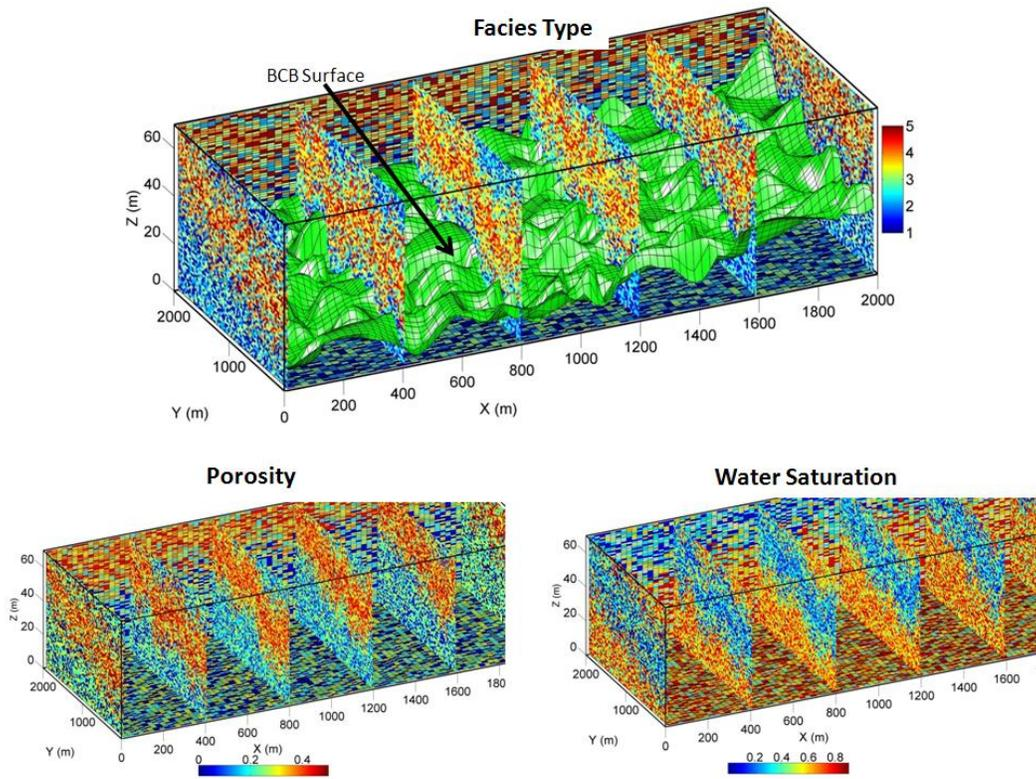
**Figure 6:** A 3D geological realization of reservoir variables. All data are the volume data. For illustration purposes different slices of the data is shown.
