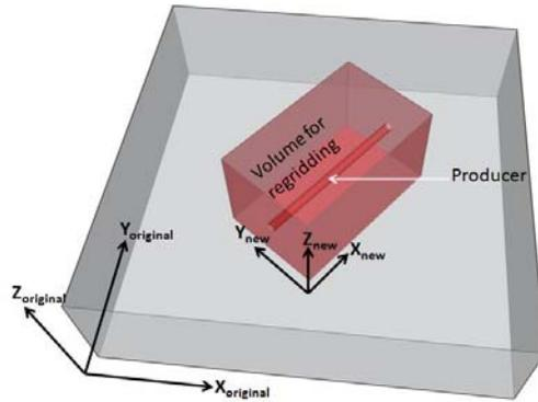
**Figure 3:** Regriding the original data along the well pair direction. Only data inside the smaller cuboid is included in the calculations.
