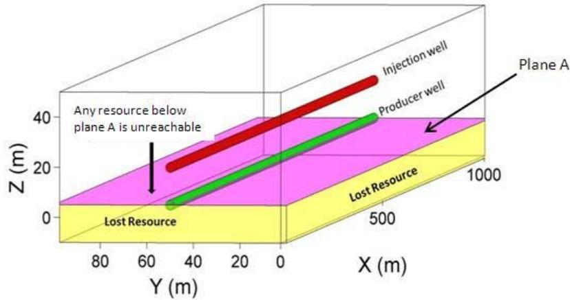
Figure 1: A well pair in SAGD. Any resource beneath producer is not accessible.
