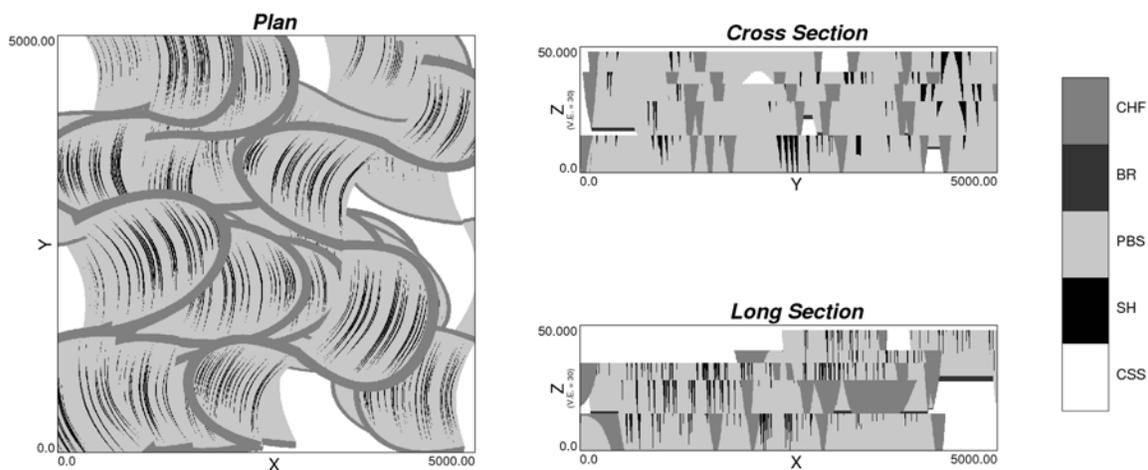
Figure 4: Three rasterized sections of training image for case 2-2-2-2-2 (vertical sections are exaggerated 30 times).
