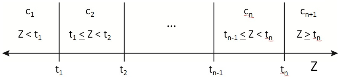
Figure 5: Illustration of classifications, c_i , relative to classification thresholds, t_j .
