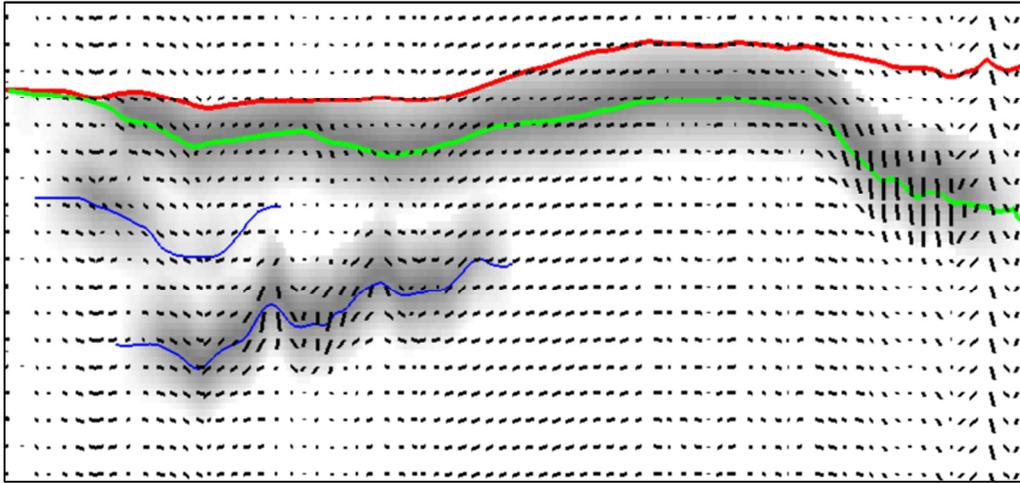
**Figure 1:** LVA field from surfaces. The intermediate surfaces only have influence around their respective areas. LVA orientation is a vertical average of all dips of each surface inversely weighted by the distance to the surface. Unit distances assumed. Note that some orientations seem off as the surface dips sharply into the page in some areas (2D slice of the 3D LVA field shown).
