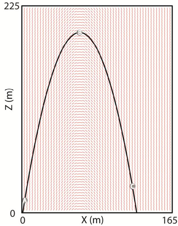
**Figure 3:** Typical cross section of the LVA field. Interpreted polylines from Figure 2 (gray intersections A, B, C) are fit with a parabola to determine the exhaustive LVA orientation.
