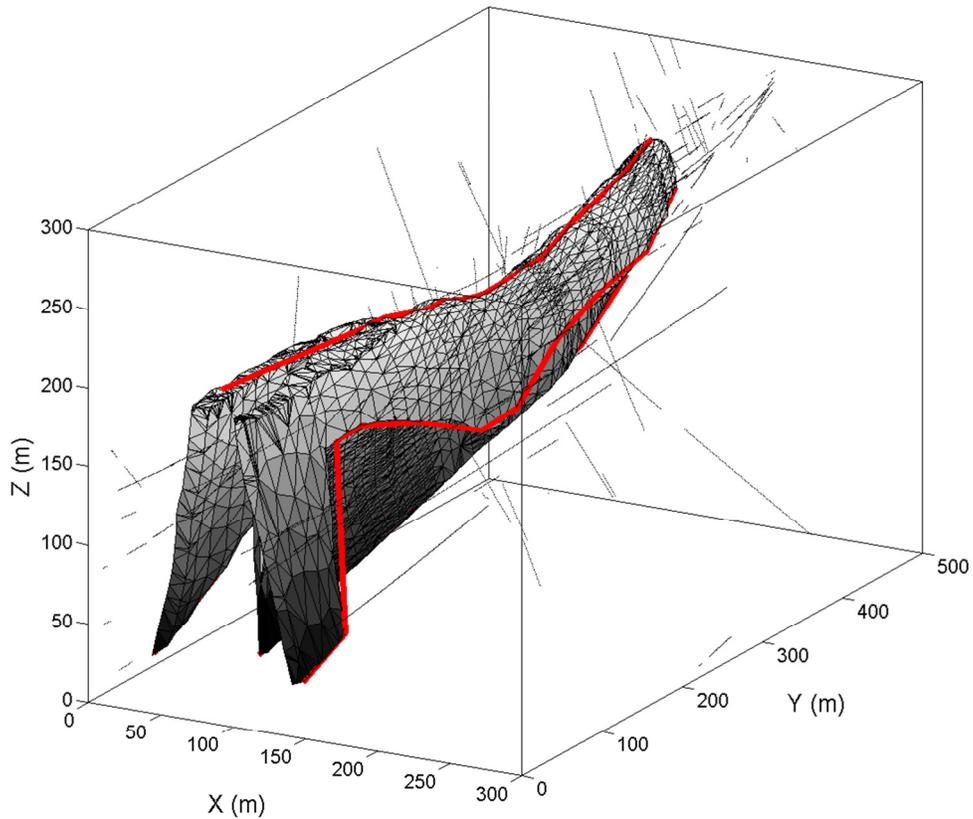
**Figure 2:** Newmont's deterministic solid. Three polylines fit to the limbs and hinge for LVA field generation.
