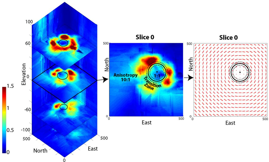
**Figure 4:** Left: Multiple slices of the block kriging map used to generate the LVA field. Middle: For each slice the LVA field is 1:1 inside the circle (defined manually for each slice) and 10:1 outside. Right: The LVA field. Length of the line is proportional to the anisotropy ratio.
