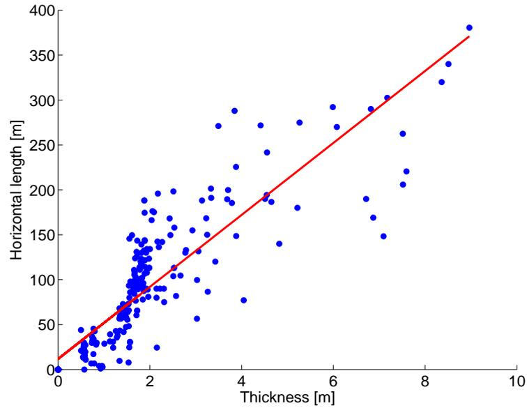
**Figure 4:** Lateral extension of barriers versus thickness.
