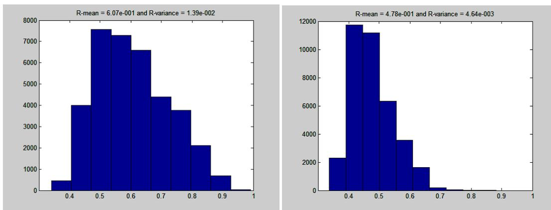
Figure 11 Comparison of reliabilities (gradient based method on the left, pca based method on the right).
