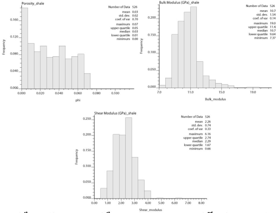
Figure 8. Porosity (1<sup>st</sup> row-left), Bulk Modulus (1<sup>st</sup> row-right) and Shear Modulus (2<sup>nd</sup> row) Histograms for Shale Facies.
