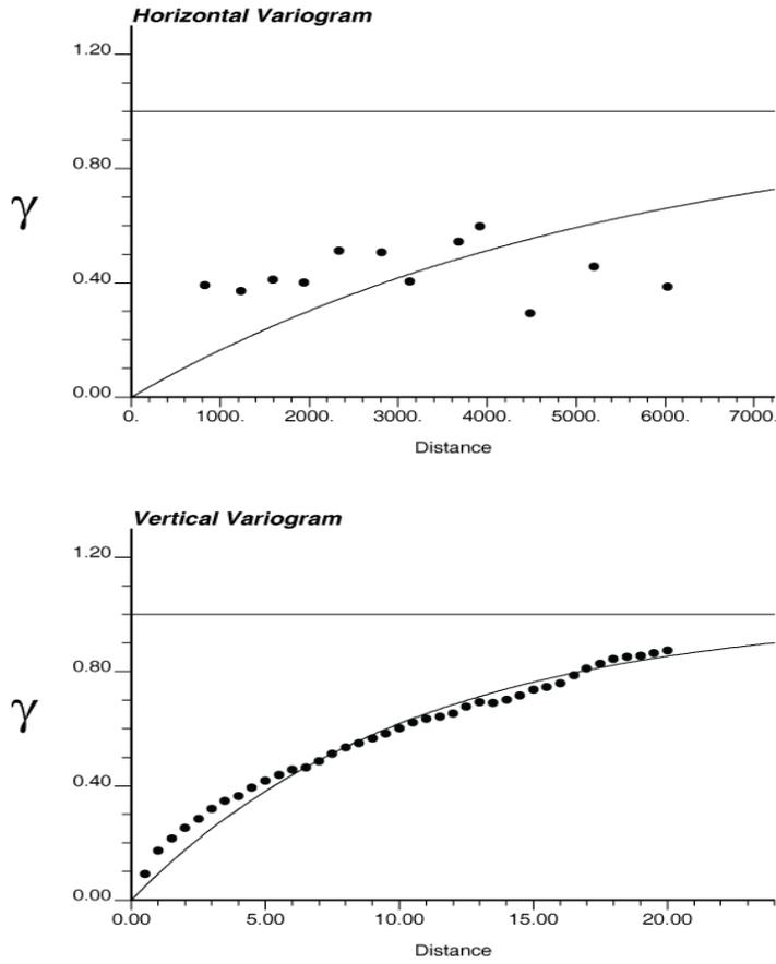
Figure 11. Horizontal (Top) and Vertical (bottom) variograms used for Porosity (sand facies) modeling.
