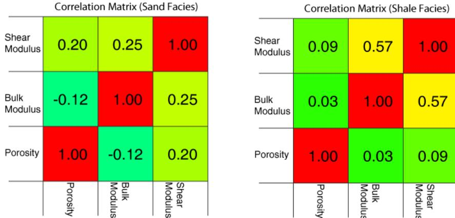
Figure 3. Correlation coefficient matrices for sand (left) and shale (right) facies.
