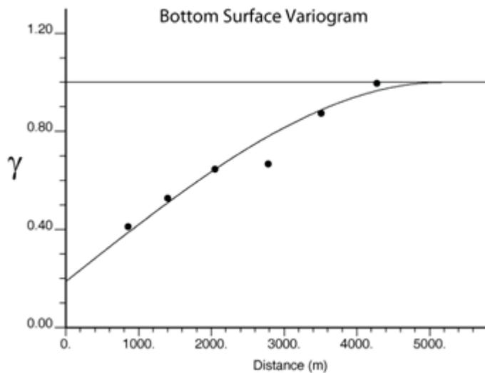
Figure 5. Experimental and fitted theoretical variogram of McMurray bottom surface.
