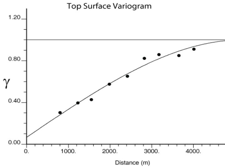
Figure 4. Experimental and fitted theoretical variogram of McMurray top surface.
