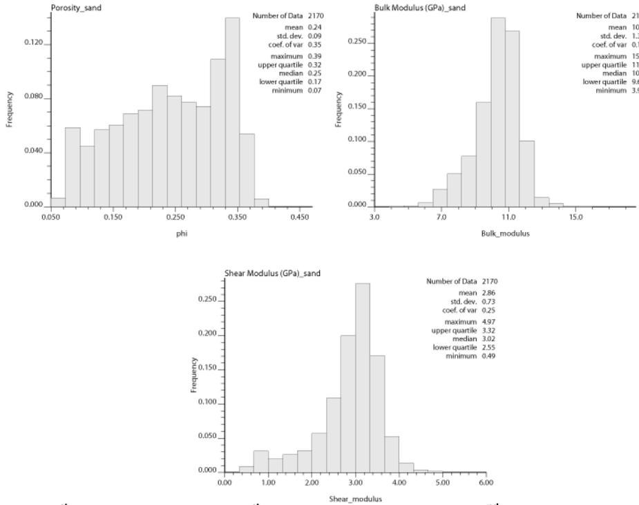
Figure 7. Porosity (1<sup>st</sup> row-left), Bulk Modulus (1<sup>st</sup> row-right) and Shear Modulus (2<sup>nd</sup> row) Histograms for Sand Facies.
