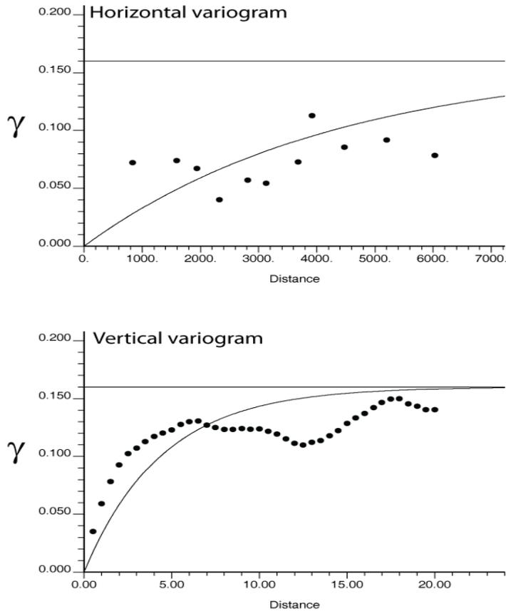
Figure 9. Horizontal (Top) and Vertical (bottom) indicator variograms used for facies modeling.
