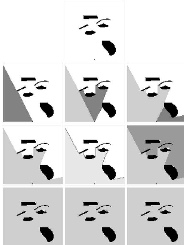
**Figure 1:** Schematics illustrating the process of determining the connected cells using line-of-sight. Black cells are non-net, white cells are net which have not been identified as visible. Varying shades of gray indicate visible cells, boundary cells, and the stages of steam chamber growth.
