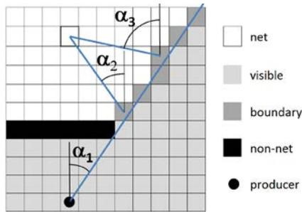
Figure 4: Illustration of angle-from-vertical for locations requiring more than one step to reach the producer.
