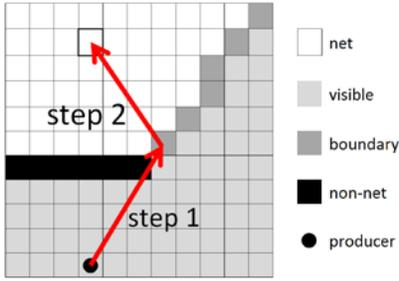
Figure 2: Illustration of the number of steps required for the bitumen to travel to the production well.
