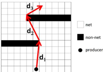
Figure 5: Illustration of the calculation of the length of the flow path.
